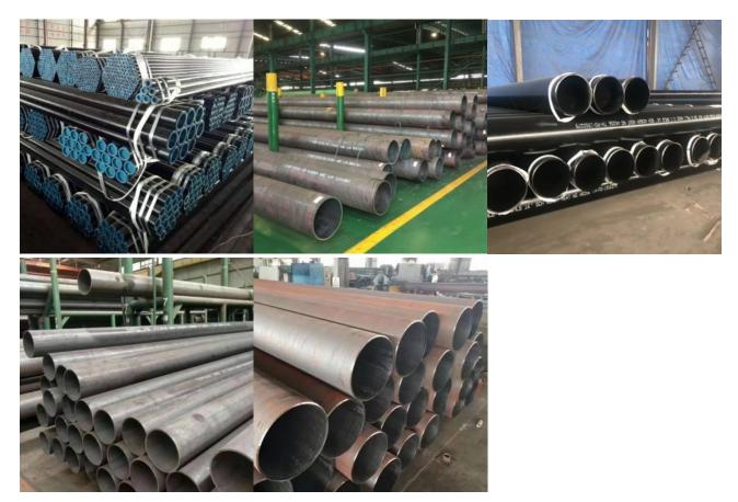
The hot expanding steel pipe is hot expanded seamless pipes, which is relatively low density but the contraction of the strong steel pipe (seamless pipe) can be referred to as thermal expansion. A process of skew rolling or drawing method to expand the pipe diameter. Steel pipe thickening in a short period of time, can produce non-standard and special types of seamless tubes with low-cost and high production efficiency, the current international developments in the field of tube rolling.
