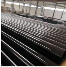
Precision seamless pipe is a pipe material producing by a cold drawn process with high precision and high-quality finish. Due to the characteristics of high-precision, in precision machinery manufacturing, auto parts, hydraulic cylinders, construction (steel sleeve) industry has a very wide range of applications.
